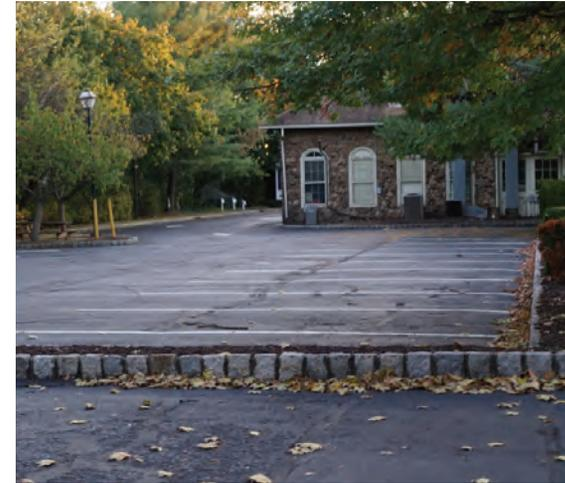
A rain garden can be installed north of the building to capture, treat, and infiltrate stormwater runoff from the rooftop of the building. Additionally, pervious pavement can be installed in the northeast parking lot to capture stormwater from the parking lot. A preliminary soil assessment suggests that more soil testing would be required before determining the soil's suitability for green infrastructure.
